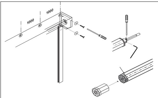
**9** Fit the shutter box using the recommended fixings and spacings. Once the shutter box has been installed check the dummy end making sure that it is securely located within the axle. If the dummy end is a shaft bolt design make sure that the centre shaft is fixed in place so that it can not slide back into the axle.
