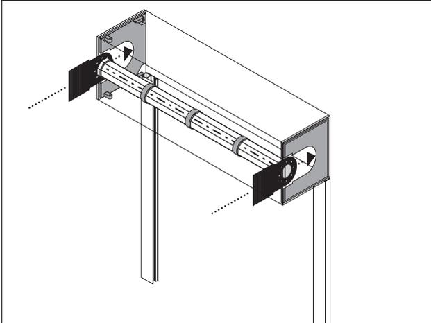
**1** Slide the axle assembly into the shutter box as shown.
