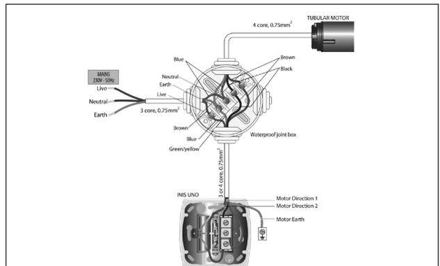
**17** Wire the control method supplied to the shutter (see section 11 for further details). If an anti-drop brake has been supplied with a limit switch (wire attached to the anti-drop brake) this will also require wiring in at this stage (see section 13.1).
