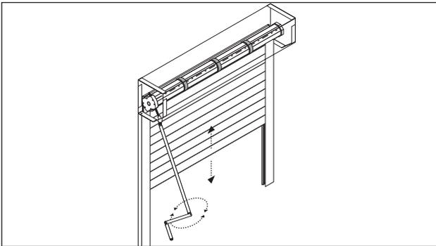
**13** Insert the crank handle temporarily and slowly wind the handle to test the operation of the shutter. Test the shutter to ensure that the curtain locks correctly when the curtain closes fully. Please refer to the operating and maintenance instructions supplied for the correct method for operating and locking the shutter. Ensure that the shutter moves freely up and down in the guide rails.
