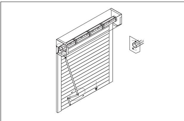
**11** The crank gear contains a stop to prevent the shutter from being overwound when it reaches the bottom. Wind the crank gear to the bottom stop then wind back  $\frac{1}{2}$  a turn.
