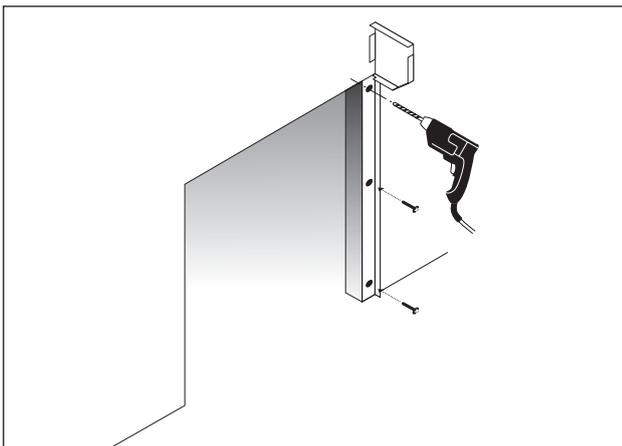
**3** Offer angle up and fix to wall ensuring vertical (use all fixing holes provided)
