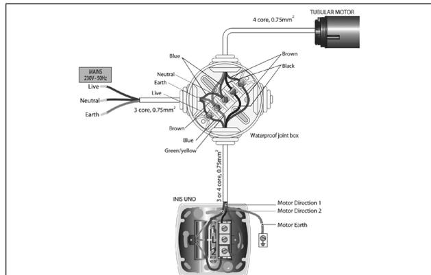
**19** Wire the control method supplied to the shutter (see section 11 for further details). If an anti-drop brake has been supplied with a limit switch (wire attached to the anti-drop brake) this will also require wiring in at this stage (see section 13.1).
