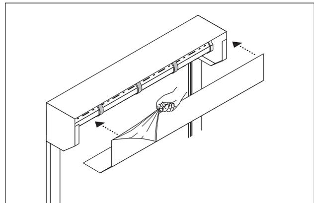
**17** Remove the protective film from the box lid then fit the box lid to the shutter box. If the shutter is externally fitted the box lid should be fastened using appropriately coloured 4mm rivets.
