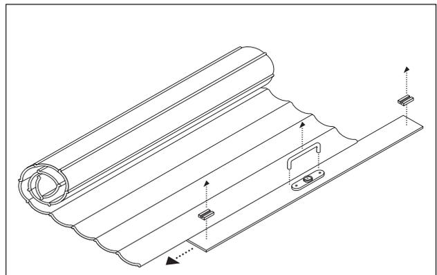
**4** Remove the stops and handles which are attached to the bottom slat then attach the bottom slat to the curtain.
