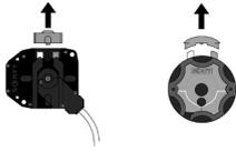
2. Remove the protective cap from the head of the motor.
