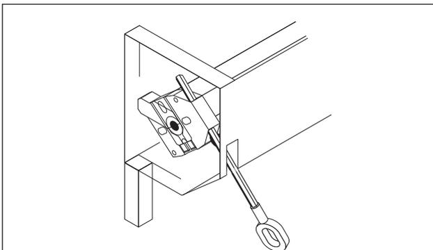
**16** If applicable attach the override handle / rigid eye / drop eye to the shutter and test the manual override facility. Once you have identified which direction will open the shutter attach the label supplied to the override handle showing the end user which direction to wind the manual override to operate the shutter.
