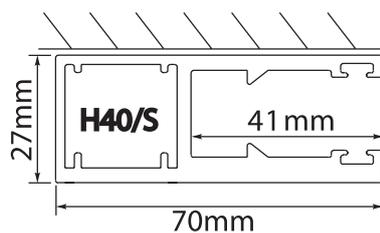
On the base of the guide rails there will be steel reinforcement plates which are part of the insurance approved specification. The type supplied will be dependant on whether the guide rails are face or reveal fitted.
