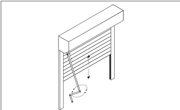
**18** If applicable attach the override handle / rigid eye / drop eye to the shutter and test the manual override facility. Once you have identified which direction will open the shutter attach the label supplied to the override handle showing the end user which direction to wind the manual override to operate the shutter.
