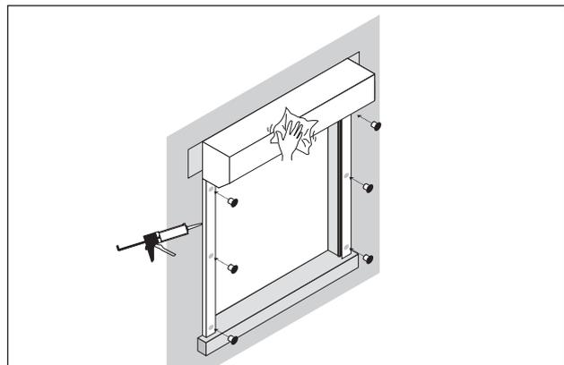
**21** To complete the installation you should fit cover caps to the guide rails (if applicable), mastic around the edges of the shutter then give the shutter a final clean and tidy.
