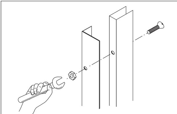
**1** The channels are supplied with the angles attached these must be removed. If 30mm x 30mm packer box has also been attached this should also be removed. Please make a note of which sides the 30x30 box section was attached to as you will need to reattach it to the correct side in step 7.
