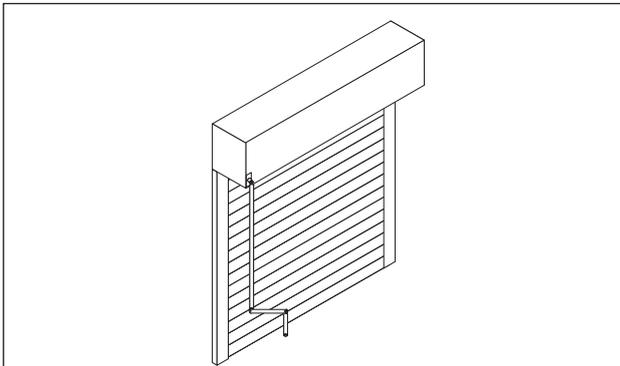
**13** If applicable attach the override handle / rigid eye / drop eye to the shutter and test the manual override facility. Once you have identified which direction will open the shutter attach the label supplied to the override handle showing the end user which direction to wind the manual override to operate the shutter.
