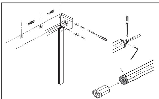
**9** Fit the shutter box using the recommended fixings and spacings. Once the shutter box has been installed check the dummy end making sure that it is securely located within the axle. If the dummy end is a shaft bolt design make sure that the centre shaft is fixed in place so that it can not slide back into the axle.
