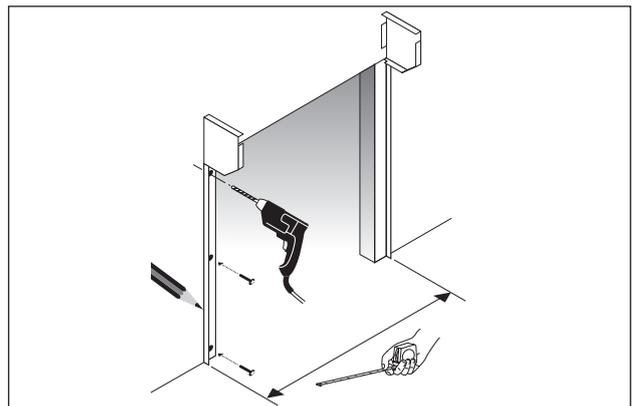
**4** Measure from the first angle to determine the position of the second angle ensuring that the angles are vertical and also that the tops of the end plates are level. Fix the angle to the wall.
