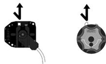
4. Identify the UP limit switch push button. Press the control switch to the UP direction until the required position is reached then turn the switch OFF.
