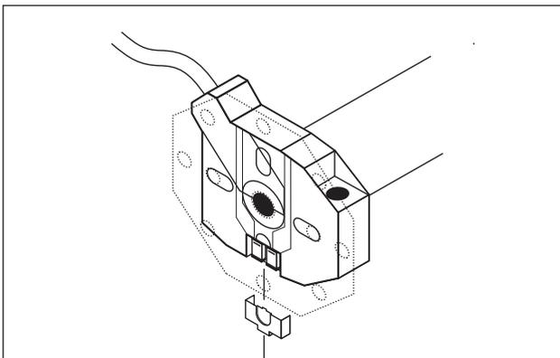
**16** Set the motor limits (see section 12). Please note that the lower motor limit should be set at a point where it is impossible to raise the curtain when the bottom lock is not engaged.
