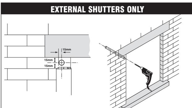
**5** Mark and drill the rod crank hole. Refer to step 6 to determine the angle of the crank hole. Please note the shutter box is not shown in this diagram. The location of the hole is determined by the exit hole in the shutter box. Drill a 10mm pilot hole followed by a 22mm hole for the tube.
