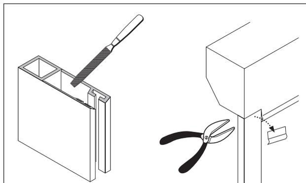
**2** File the top of the guides at an angle to create the optimum lead in for the curtain. Guide insert should also be trimmed to suit the filed guide tops. If the shutter is being face fitted remove the lip from the box back which overlaps the guide rails.
