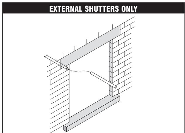
**6** Cut belt tube to correct length and insert
