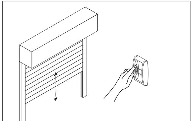
**14** Test the operation of the shutter to ensure that the shutter moves freely up and down in the guide rails and that the shutter stops at its preset fully open and fully closed limits. If a remote control has been supplied with safety devices these should also be checked at this stage.
