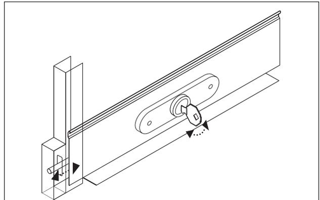
**8.** If a lock has been supplied in the bottom slat you should remove the bottom slat from the curtain. Slide the bottom slat down into the guide rails and check that the lock bars in the bottom slat will locate into the prepared guide rail keeps. Enlarge the keeps if necessary.
