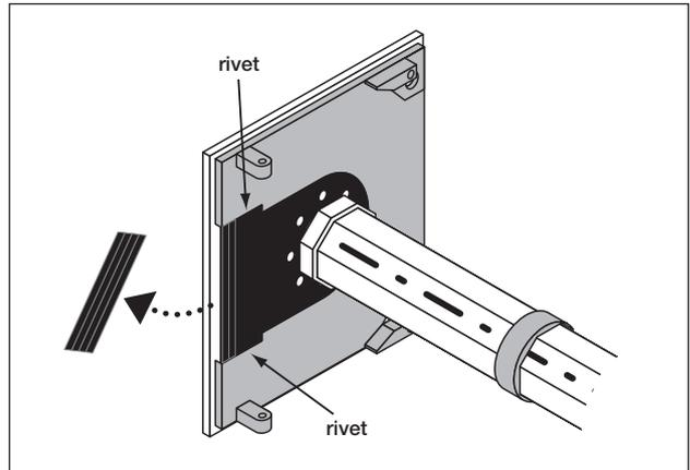
**2** Remove the excess material from the axle supports as shown then rivet the black axle supports in place.
