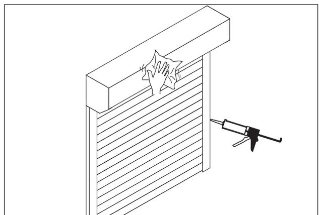
**17** To complete the installation you should mastic around the edges of the shutter then give the shutter a final clean and tidy.
