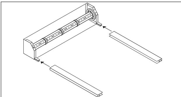
**3** Carefully locate the guide rails fully onto the box lugs ensuring that on face fit guides the 13mm holes are on the outside. When moving the shutter as a complete unit you should minimise the movement of the guide rails to prevent the locating lugs from being snapped off the shutter box. If the shutter is too large to be lifted up as a complete unit you should offer up, locate and fix the individual guide rails then the shutter box.
