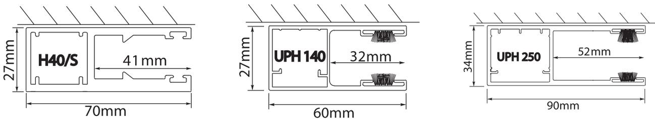
Certain guide rails have an internal and external face, due to their extrusion profile. These guide rails must be installed the correct way round. Please check the guide rails you have been supplied before you begin installing the shutter.
