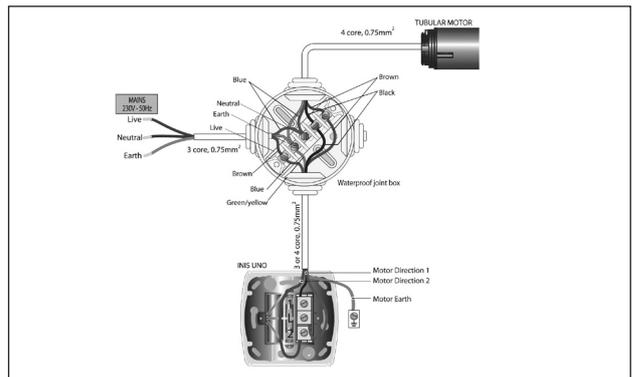
**10** Wire the control method supplied to the shutter (see section 11 for further details). If an anti-drop brake has been supplied with a limit switch (wire attached to the anti-drop brake) this will also require wiring in at this stage (see section 13.1).
