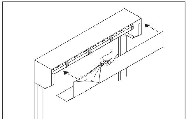
**18** Remove the protective film from the box lid then fit the box lid to the shutter box. If the shutter is externally fitted the box lid should be fastened using appropriately coloured 4mm rivets.
