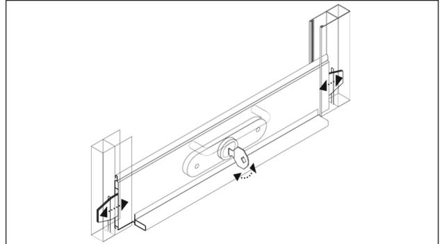
**8** If shoot bolts or a lock have been supplied in the bottom slat you should remove the bottom slat from the curtain. Slide the bottom slat down into the guide rails and check that the lock bars in the bottom slat will locate into the prepared guide rail keeps. Enlarge the keeps if necessary.
