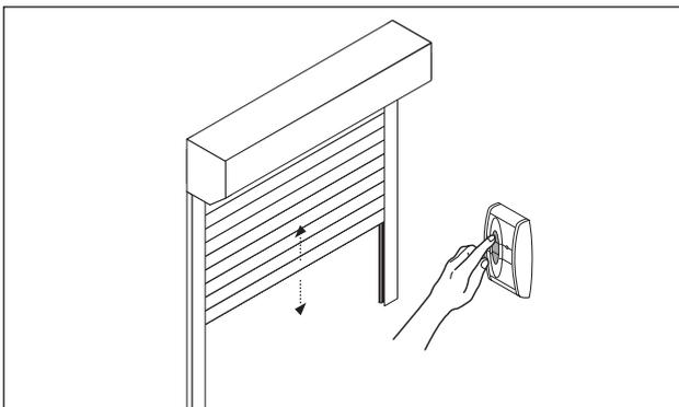
**20** Test the operation of the shutter to ensure that the shutter moves freely up and down in the guide rails and that the shutter stops at its preset fully open and fully closed limits. If a remote control has been supplied with safety devices these should also be checked at this stage. Also ensure that the locks engage and disengage satisfactorily.
