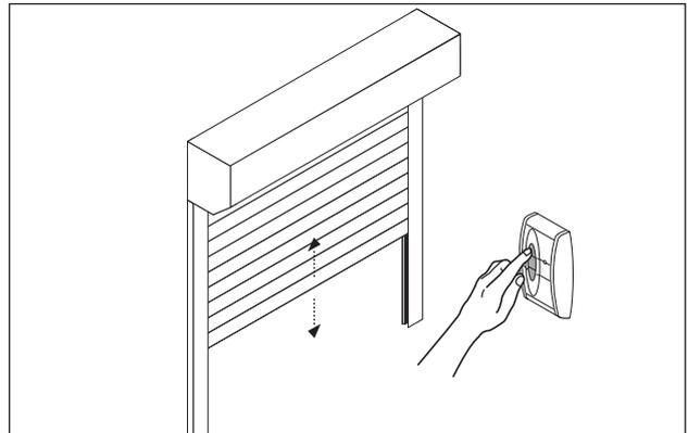
**20** Test the operation of the shutter to ensure that the shutter moves freely up and down in the guide rails and that the shutter stops at its preset fully open and fully closed limits. If a remote control has been supplied with safety devices these should also be checked at this stage.
