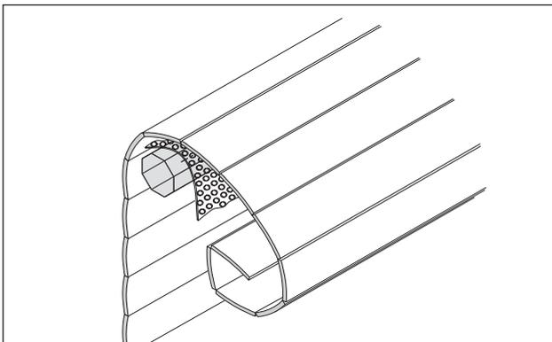
**⚠ RISK OF MATERIAL DAMAGE!** **13** Cover the axle with bubble wrap or a similar material to prevent the curtain from being damaged during the curtain loading process. Carefully load the curtain over the axle.
