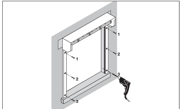
**8** Starting with the top holes, fix the guide rails ensuring that the guide rails are vertical and that the shutter box is horizontal. Use the fixings recommended on page 8. 7mm hole right through then front hole enlarged to 13mm.
