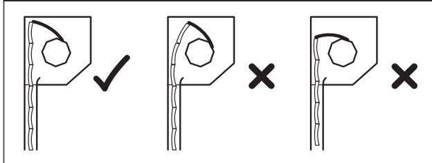
**11** Check the curtain height. When pushed towards the back of the shutter box the curtain should finish just under the box top. If the curtain is too tall then slats should be removed to obtain the correct height. If the curtain finishes more than one slat beneath the shutter box top then the curtain is too short and the height must be increased in order for the shutter to lock correctly when fully down.
