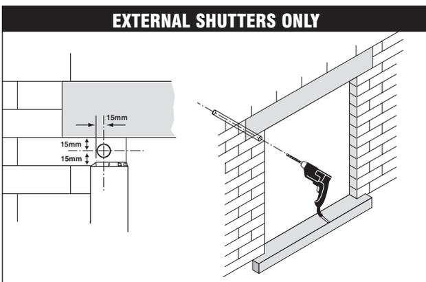
**5** Mark and drill the belt tube hole. Drill a 10mm pilot hole followed by a 22mm hole for the tube.
