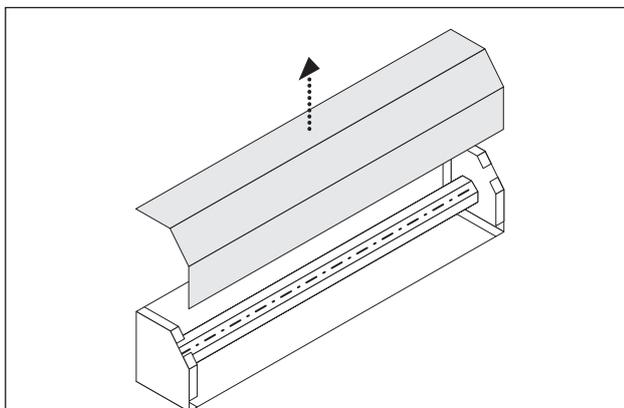
**1** Remove the lid from the shutter box. If attached remove locking springs / attachment straps from the axle and keep safe for step 12.
