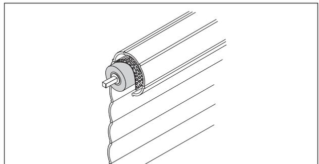
**! RISK OF MATERIAL DAMAGE!** **10** Cover the axle with bubble wrap or a similar material to prevent the curtain from being damaged during the curtain loading process. Carefully load the curtain over the axle.
