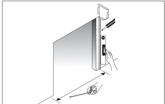
**2** Measure the opening to determine the location of the first length of angle. If the floor is sloping you must fit the higher side first. Fix the angle to the wall.
