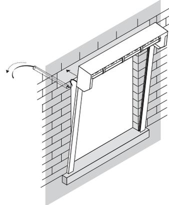
**8** Unwind belt and feed through tube whilst offering the shutter to the opening
