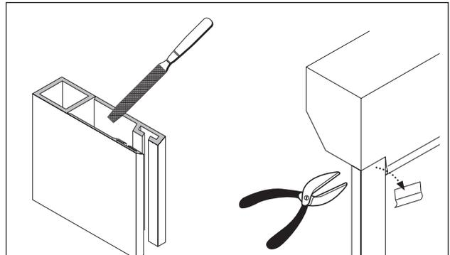
**2** File the top of the guides at an angle to create the optimum lead in for the curtain. Guide insert should also be trimmed to suit the filed guide top and securely crimped in place. If the shutter is being face fitted remove the lip from the box back which overlaps the guide rails.
