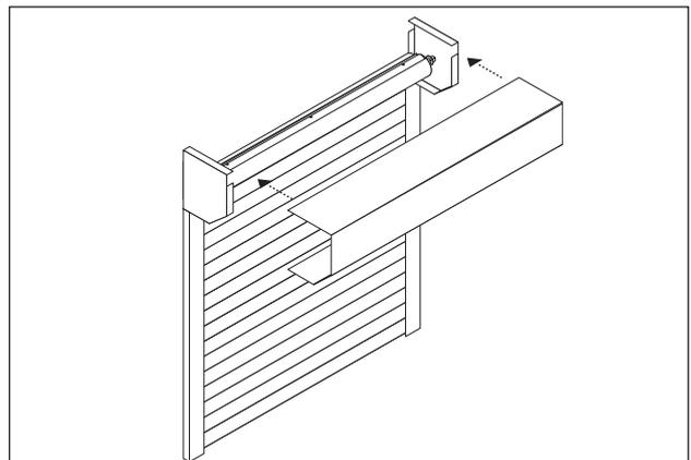
**15** If required fit the hood / fascia. If the shutter is externally fitted the hood / fascia should be fastened using appropriately coloured 4mm rivets.
