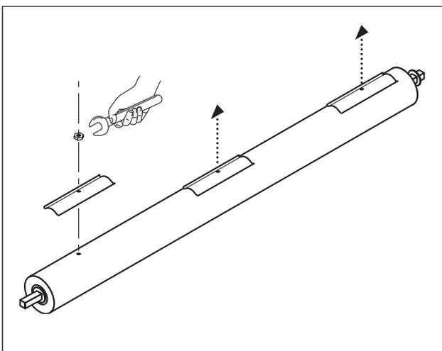
**5** Remove the attachment strips from the axle.
