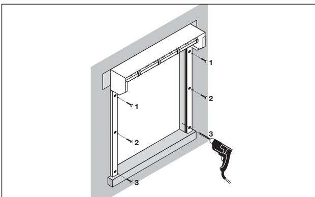
**9** Starting with the top holes, fix the guide rails ensuring that the guide rails are vertical and that the shutter box is horizontal. Use the fixings recommended on page 8. 7mm hole right through then front hole enlarged to 13mm.
