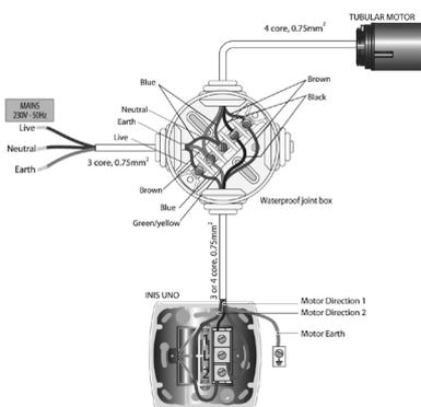
**17** Wire the control method supplied to the shutter (see section 11 for further details). If an anti-drop brake has been supplied with a micro limit switch (wire attached to the anti-drop brake) this will also require wiring in at this stage (see section 13.1).
