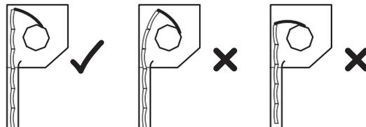
**14** Check the curtain height. When pushed towards the back of the shutter box the curtain should finish just under the box top. If the curtain is too tall then slats should be removed to obtain the correct height. If the curtain finishes more than one slat beneath the shutter box top then the curtain is too short and the height must be increased in order for the shutter to lock correctly when fully down.
