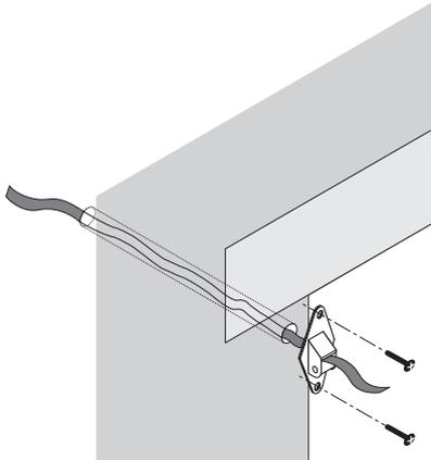
**19** Slide roller on belt and mount on the internal wall.
