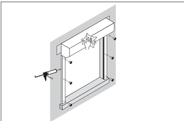
**21** To complete the installation you should fit cover caps to the guide rails (if applicable), mastic around the edges of the shutter then give the shutter a final clean and tidy.
