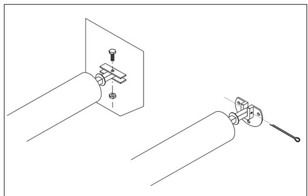
**6** Attach the axle to the end plates using the fixings provided. You must ensure that the bolts located along the length of the axle for curtain attachment will be available for step 11.
