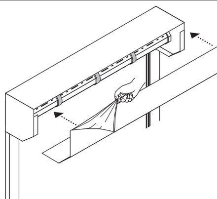
**17** Remove the protective film from the box lid then fit the box lid to the shutter box. If the shutter is externally fitted the box lid should be fastened using appropriately coloured 4mm rivets.
