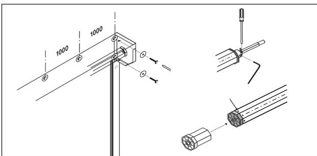
**9** Fit the shutter box using the recommended spacings. The minimum required fasteners are No.12 x 2½" screws and plugs for masonry and M8 fasteners with 10mm engagement for steel. A minimum of 2 fixings per end plate are required. Once the shutter box has been installed check the dummy end making sure that it is securely located within the axle. If the dummy end is a shaft bolt design make sure that the centre shaft is fixed in place so that it can not slide back into the axle.
