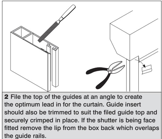
**2** File the top of the guides at an angle to create the optimum lead in for the curtain. Guide insert should also be trimmed to suit the filed guide top and securely crimped in place. If the shutter is being face fitted remove the lip from the box back which overlaps the guide rails.
