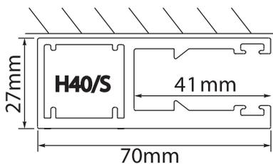
Certain guide rails have an internal and external face, due to their extrusion profile. These guide rails must be installed the correct way round. Please check the guide rails you have been supplied before you begin installing the shutter.
