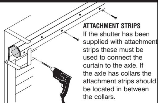
**12** Attach the curtain directly to the axle through the top two slats using the screws provided. Do not use locking springs. Screw heads must be countersunk to prevent damage to the curtain.
