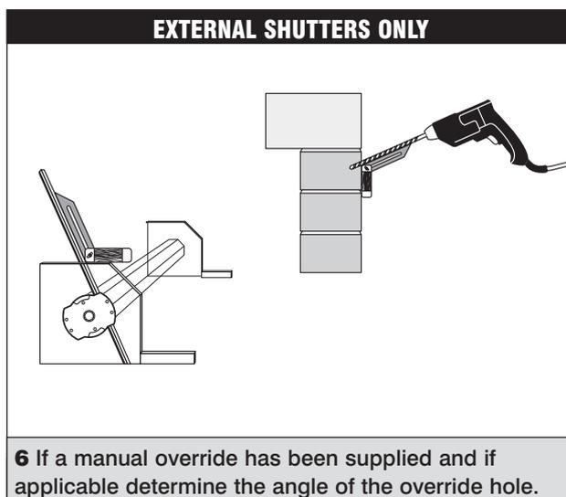
**6** If a manual override has been supplied and if applicable determine the angle of the override hole.
