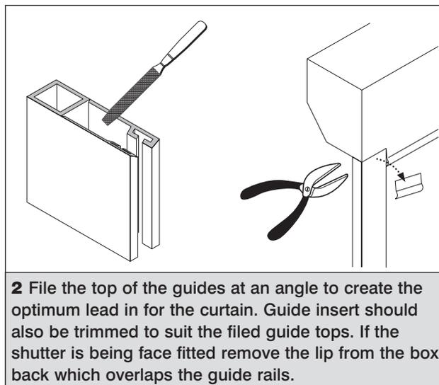
**2** File the top of the guides at an angle to create the optimum lead in for the curtain. Guide insert should also be trimmed to suit the filed guide tops. If the shutter is being face fitted remove the lip from the box back which overlaps the guide rails.
