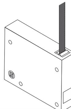
**22** Load the belt into the winder. The belt will be supplied to the correct length. Take off the front of the winder, pass the belt between the rollers and fasten by knotting securely into the centre of the large cog. Reassemble the winder before fastening to the wall.
