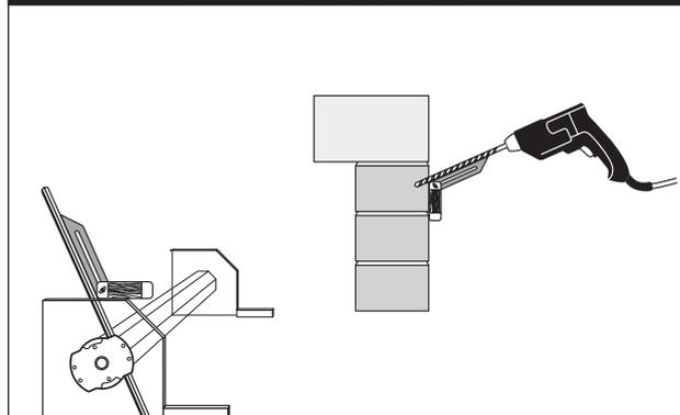
**6** If a manual override has been supplied and if applicable determine the angle of the override hole.
