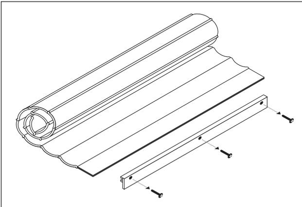
**3** If a bottom slat handle has been fitted to the curtain it should be removed before you attempt to load the curtain into the shutter.
