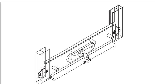
**10** If a lock has been supplied in the bottom slat you should remove the bottom slat from the curtain. Slide the bottom slat down into the guide rails and check that the lock bars in the bottom slat will locate into the prepared guide rail keeps. Enlarge the keeps if necessary.
