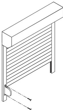
**23** Mount the winder at a convenient height for operation either to the wall or to the guide rails as appropriate.
