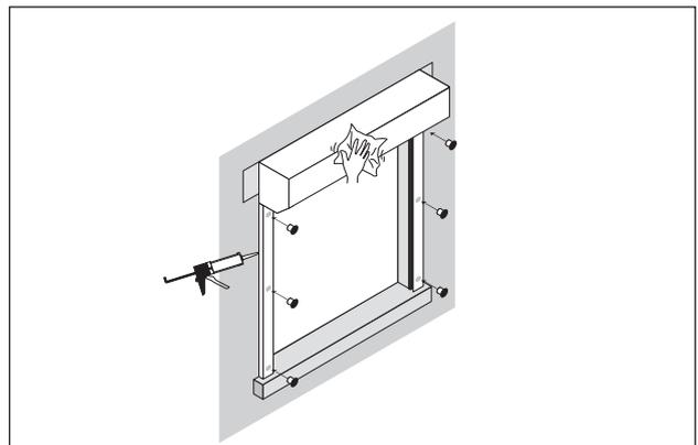
**16** To complete the installation you should fit cover caps to the guide rails (if applicable), mastic around the edges of the shutter then give the shutter a final clean and tidy.
