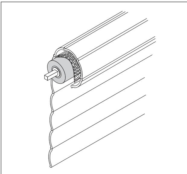
**9** Large curtains will be supplied in two or more sections to enable them to be transported. There are two alternative methods for assembling the curtain:
