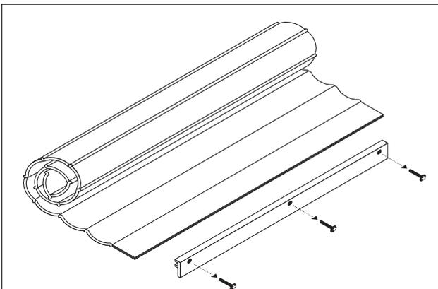
**5** If a bottom slat handle has been fitted to the curtain it should be removed before you attempt to load the curtain into the shutter.
