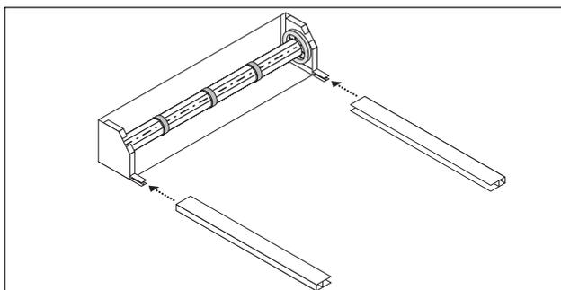
**3** Carefully locate the guide rails onto the box lugs ensuring that on face fit guides the 13mm holes are on the outside. When moving the shutter as a complete unit you should take care to prevent the lugs being snapped off the box ends by the leverage available from the guide rails. If the shutter is too large to be lifted up as a complete unit you should offer up, locate and fix the individual guide rails then the shutter box.
