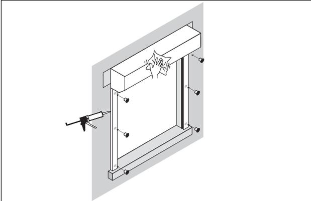
**18** To complete the installation you should fit cover caps to the guide rails (if applicable), mastic around the edges of the shutter then give the shutter a final clean and tidy.
