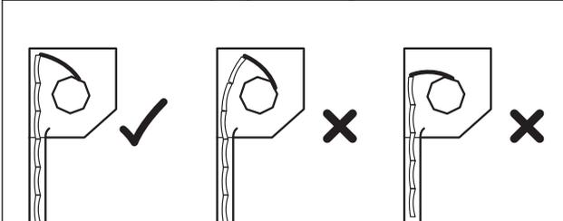
**5** Check the curtain height. When pushed towards the back of the shutter box the curtain should finish just under the box top. If the curtain is too tall then slats should be removed to obtain the correct height. If the curtain finishes more than one slat beneath the shutter box top then the curtain is too short and the height must be increased in order for the shutter to lock correctly when fully down.
