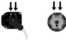
3. Fully depress both limit switch push buttons. They will automatically lock in the down position. Operate the control switch and check the direction of rotation. If it is incorrect, turn the switch OFF, reverse the black and brown motor direction wires and try again.
