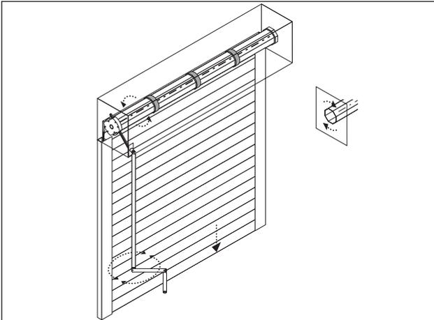
**5** Wind the crank gear to the bottom stop then wind the axle back ½ a turn.
