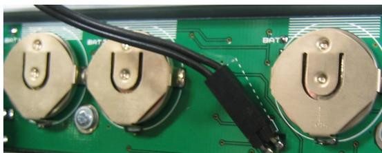
Feed the wire through the bottom slat transmitter rubber seal then attach to the connector.
