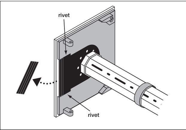
**2** Remove the excess material from the axle supports as shown then rivet the black axle supports in place.
