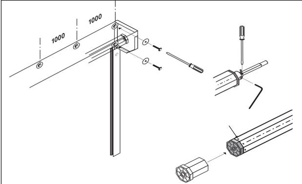
**7** Fit the shutter box using the recommended fixings and spacings. Once the shutter box has been installed check the dummy end making sure that it is securely located within the axle. If the dummy end is a shaft bolt design make sure that the centre shaft is fixed in place so that it can not slide back into the axle.
