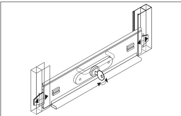
**3** If shoot bolts or a lock have been supplied in the bottom slat you should remove the bottom slat from the curtain. Slide the bottom slat down into the guide rails and check that the lock bars in the bottom slat will locate into the prepared guide rail keeps. Enlarge the keeps if necessary.
