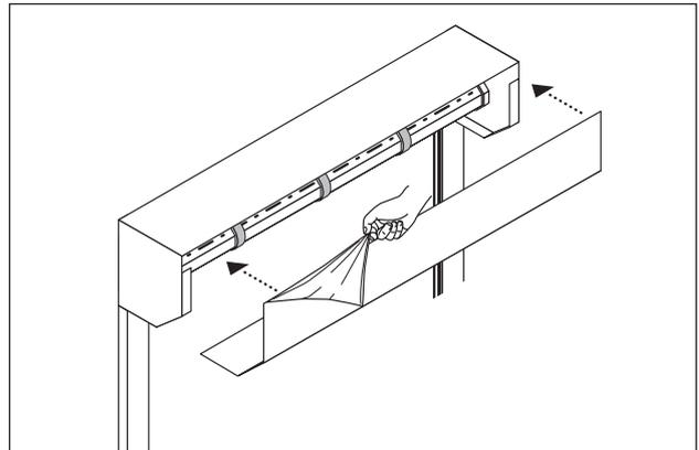
**14** Remove the protective film from the box lid then fit the box lid to the shutter box. If the shutter is externally fitted the box lid should be fastened using appropriately coloured 4mm rivets.
