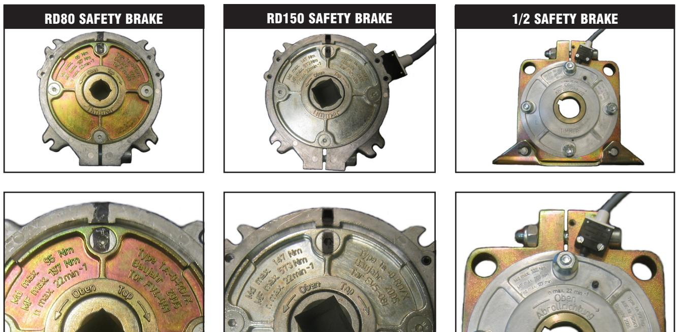
If after activation you are unable to reset the brake as shown above you will need to reorder a replacement brake, which will be chargeable. Once you have swapped the brakes over the activated brake should be returned to your supplier for inspection. As long as the safety brake has not been damaged the brake will be reset and returned to you for use as a spare.
