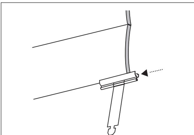
**15** Load the locking springs onto the curtain
