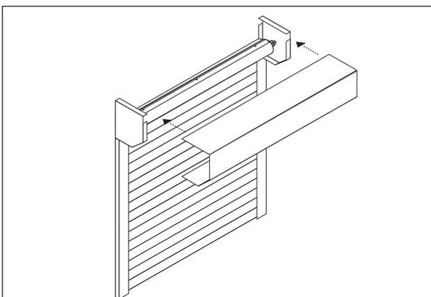
**16** If required fit the hood / fascia. If the shutter is externally fitted the hood / fascia should be fastened using appropriately coloured 4mm rivets.
