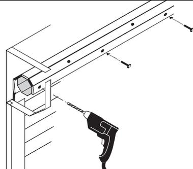
**13** Attach the curtain directly to the axle through the top two slats using the screws provided. Do not use locking springs. Screw heads must be countersunk to prevent damage to the curtain.
