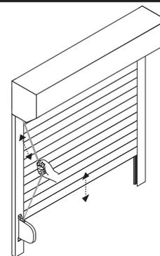
**24** Test the operation of the winder and the shutter to ensure that the belt feeds into and out of the winder correctly and also that the shutter moves freely up and down in the guide rails.
