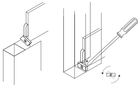
**12** If adjustable T stops have been fitted in the bottom slat they should be set to an angle of approximately 45° to enable the bottom slat to enter the top of the guide rail. Once the bottom slat has entered the guide rail the T stop should be set to the horizontal position to prevent the curtain from being accidentally lifted out of the guide rails.
