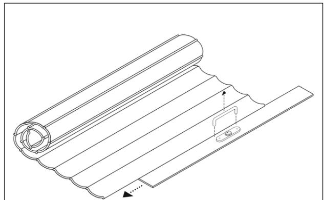
**10** To prevent damage to the shutter and the surroundings and also to make the following step easier, remove the handles and stops from the bottom slat. Reattach the bottom slat to the curtain. If necessary remove the bottom slat handle from the bottom slat.
