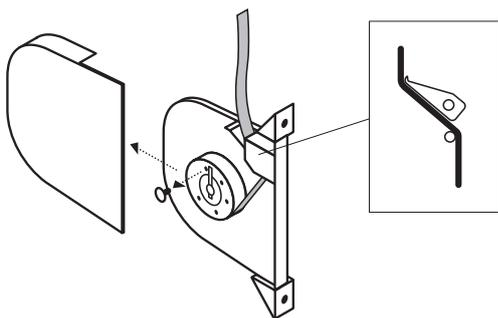
**21** Load the belt into the winder. The belt will be supplied to the correct length. Pass the belt under the metal flap and between the chrome rollers. 500mm from the end of the belt cut a 10mm lengthways slit along the centre. Hook onto the pretensioned spring casing then release.
