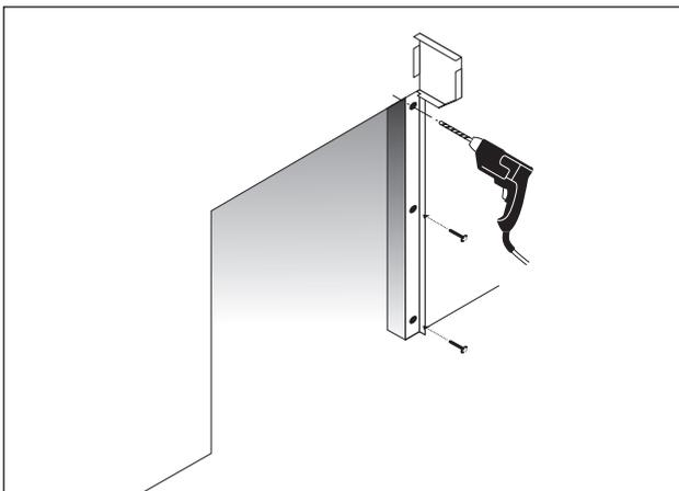
**3** offer angle up and fix to wall ensuring vertical (use all fixing holes provided)
