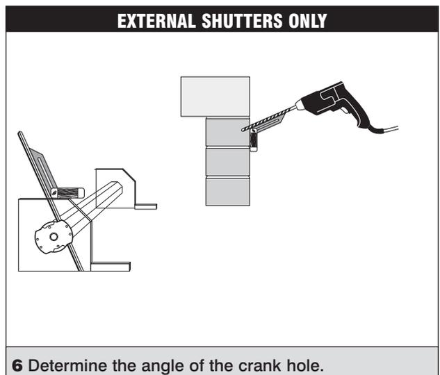
**6** Determine the angle of the crank hole.
