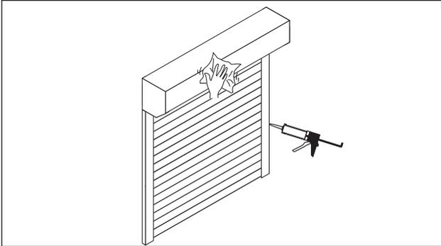
**18** Test the operation of the shutter to ensure that the shutter moves freely up and down in the guide rails and that the shutter stops at its preset fully open and fully closed limits. If a remote control has been supplied with safety devices these should also be checked at this stage. To complete the installation you should mastic around the edges of the shutter then give the shutter a final clean and tidy.
