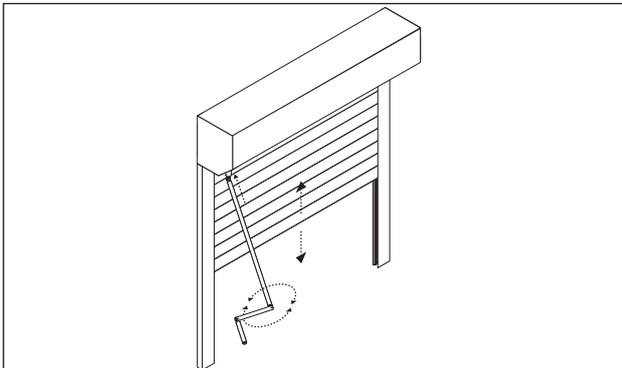
**19** If applicable attach the override handle / rigid eye / drop eye to the shutter and test the manual override facility. Once you have identified which direction will open the shutter attach the label supplied to the override handle showing the end user which direction to wind the manual override to operate the shutter.
