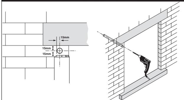
**5** If applicable mark and drill the override hole ensuring the hole is drilled at the correct angle (see step 6). Drill a 10mm pilot hole followed by a 22mm hole
