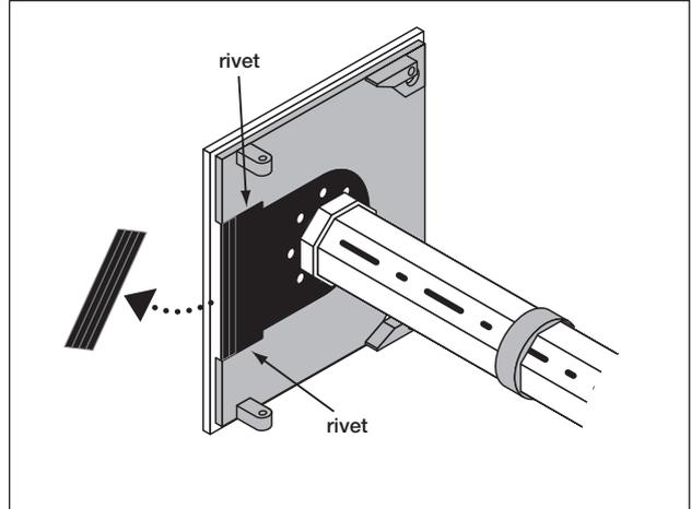
**2** Remove the excess material from the axle supports as shown then rivet the black axle supports in place.
