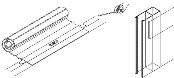
**9** If the curtain contains a lock installed in a slat above the bottom slat you will need to prepare the guide rails for the lock bar, which will protrude from the slat when the lock is operated. Measure the distance from the bottom of the curtain to the lock bar then create a hole in each guide rail to suit the lock bar.
