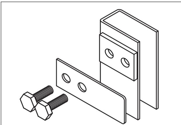
**15** Attach the stops to the guide channels (as shown above) and if applicable attach handles to the bottom slat.
