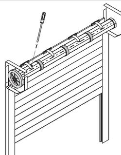
**16** Before you attach the curtain to the axle you should determine where you will mount the winder then pull the belt wrapped around the drive wheel so that the belt will pass the winder by at least 400mm. Attach the locking springs to the axle using the screws supplied.
