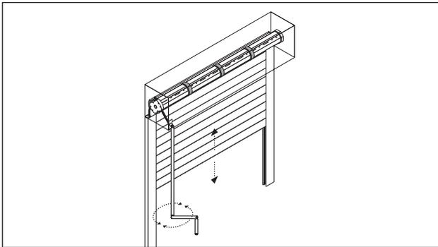
**7** Insert the crank handle temporarily and slowly wind the handle to test the operation of the shutter. Test the shutter to ensure that the curtain locks correctly when the curtain closes fully. Please refer to the operating and maintenance instructions supplied for the correct method for operating and locking the shutter. Ensure that the shutter moves freely up and down in the guide rails.
